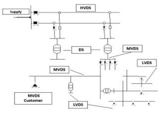
Figure 1. Representation of an electric power distribution system.
