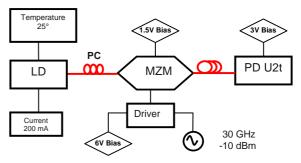
Figure 7. Photonic millimeter-wave generator based on external modulation. Components additional to Fig. 3: ILX Lightwave LDT-5412 temperature controller; Precision Current Source: ILX Lightwave LDX-3545B
