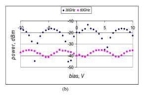
Figure 10. VPI simulations (a) and power measurements of 30 GHz and 60 GHz signals at the output of the PD (b)
