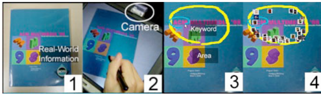
Figure 9. Combination with real-world information: Capturing real-world information as a picture (1, 2) and drawing two closed curves (3, 4). One curve (shown in yellow) means an area and the other (shown in blue) means a keyword.
