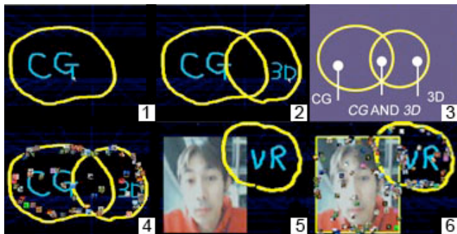
Figure 3. Drawing a Venn diagram: By continuously drawing crossed curves and keywords, a user creates a Venn diagram and can then retrieve information by forming a complex query (1, 2, 3, 4). It is possible to create a Venn diagram between a drawing and an image that contains character information (5, 6).
