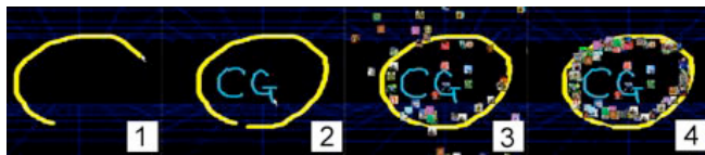
Figure 2. Rough search: A user first draws a closed curve with the area pen and a keyword inside the curve with the text pen. As the system recognizes the area and keyword, related information nodes appear inside the area.
