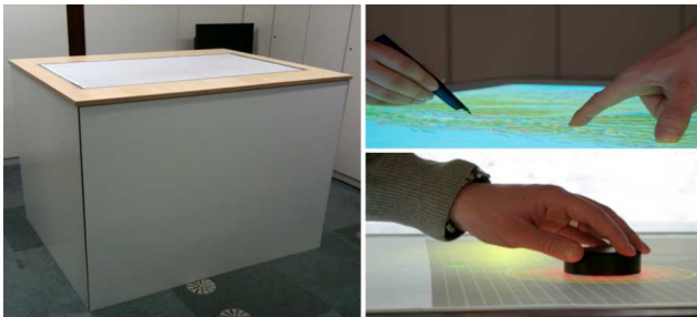
Figure 3. The useTable and its interaction possibilities (pen, multi-touch, tangible puck)
