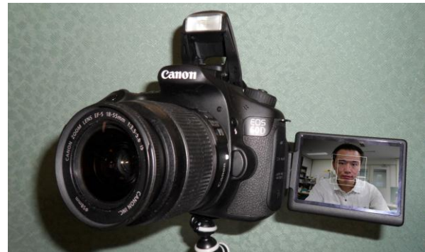
Figure 3. Canon 60D camera with foldable LCD screen and face detection.
