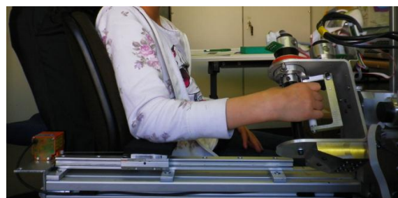
Figure 3. Handreha : The developed desktop hand rehabilitation device
