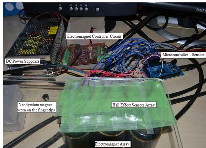
Figure 1. Haptic mouse system : User can move the neodymium magnet worn on the finger tip above the device surface and interact with the computer & sense haptic feedback for their inputs.
