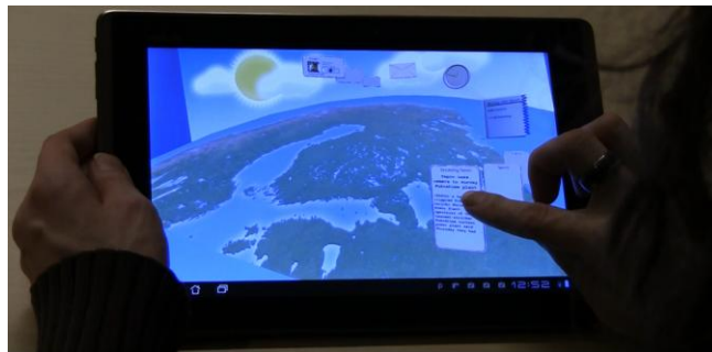
Figure 6. In a context-aware map based 3D UI prototype, a user is able to select words (e.g., Fukushima) from news feed and then drag and drop it onto the map environment for getting more information about that news.
