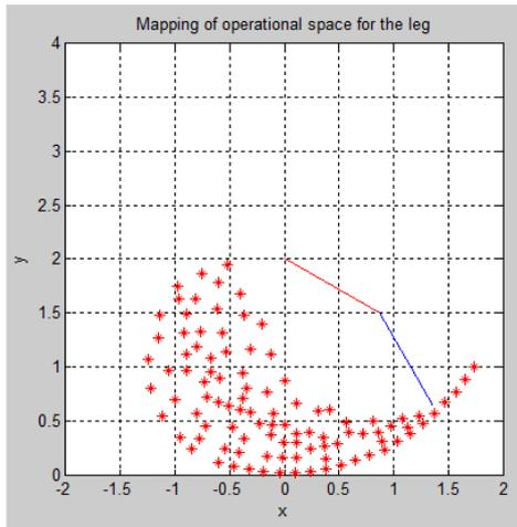
Figure 6. Mapping of the leg operation space. Strictly in this region, the FCMAC ANN can provide the desired output after training.
