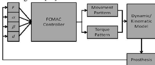
Figure 4. Proposed model to control the prosthesis [13].
