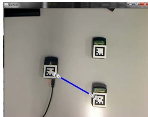
Figure 8. Displayed network connection information among sensor nodes.
