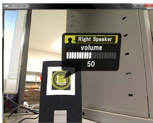
Figure 7. Volume control of right speaker with AR.
