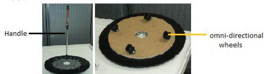
Figure 3. Hand held stick on a disc with omni-directional wheels.
