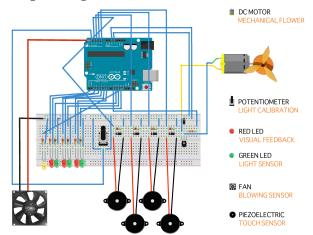
Figure 2 – Orthographic top view from the connection sketch with the input sensors and the output motor.
