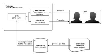
Figure 1. System architecture
