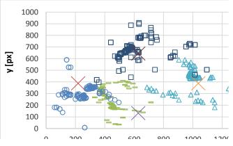
Figure 7. Calibration checker result from the Kindle tablet, the cross show the target, the other signs show the actual values
