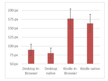
Figure 5. Mean absolute error (MAE) between the reference points and the gaze points in pixels with standard deviations
