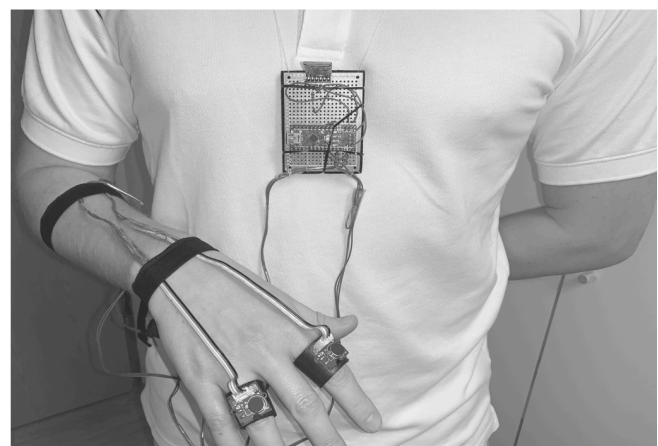
Figure 3. Haptic rings with Grove vibration motors connected to Arduino board with cables
