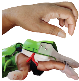
Figure 2. Image showing a stroke survivor’s hand with hyperflexion in the fingers being offset by WiGlove.
