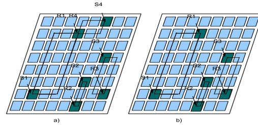
Figure 9: Hormonal loops: a) four loops out of which 2 are related i.e., loops ( $S1, R1/R4$ ) and ( $S4, R1/R4$ ) where  $R1/R4$  stands for the cell which recognises incoming *S hormones* from both cells  $S1$  and  $S4$ ; b) three unrelated loops. The cells *encoding IDs* are omitted for the sake of clarity
