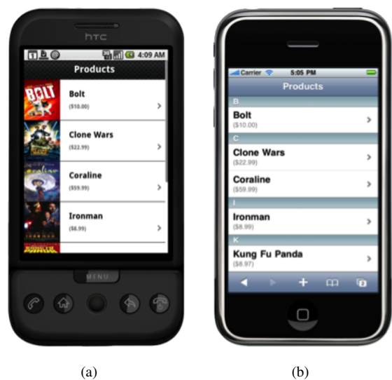
Figure 7. Adaptive mCommerce web application on two smartphones. (a) An Android smartphone, the HTC Dream and (b) an iOS smartphone, the Apple iPhone
