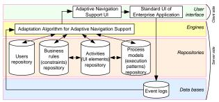
Figure 3. The architecture of the ANS component.
