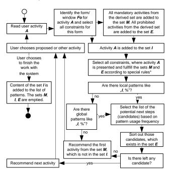
Figure 5. Simplified view of the adaptation algorithm behind the ANS.
