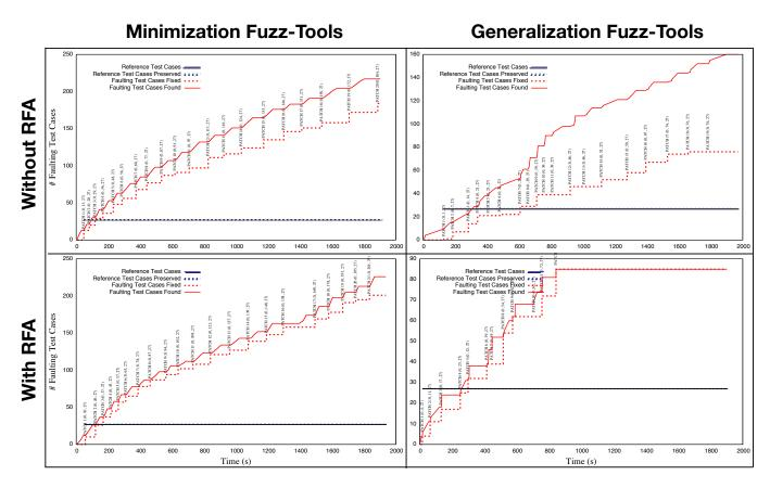
Fig. 3. Results comparing the exposure window of Retrospective Fault Analysis and minimization vs. generalization tools.
