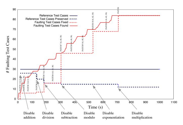
Fig. 4. FUZZBUSTER sacrifices functionality to protect the program against vulnerabilities.
