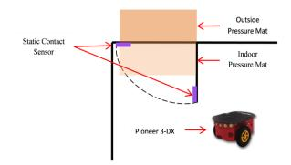
Figure 1. Hardware topology in experimental environment.
