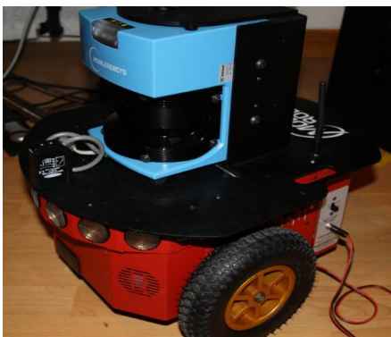
Figure 3. Pioneer P3DX mobile robot fitted with LMS 200 laser.
