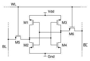
Figure 1. 6T SRAM cell
