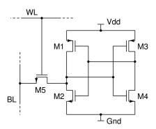
Figure 3. 5T SRAM cell
