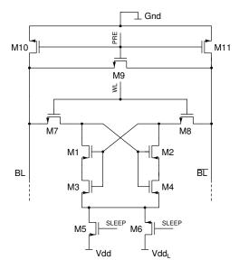
Figure 9. Modified 4T SRAM cell
