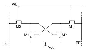
Figure 5. 4T loadless SRAM cell
