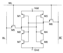
Figure 7. 6T SRAM cell with stacking
