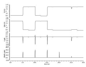
Figure 10. Power dissipation and  $I_{Leak}$  of a modified 4T SRAM cell
