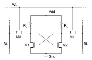
Figure 2. 4T SRAM cell
