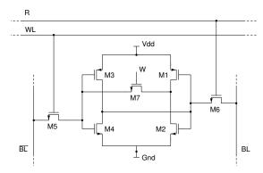
Figure 4. 7T SRAM cell
