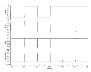
Figure 6. Power dissipation and  $I_{Leak}$  of 6T SRAM cell
