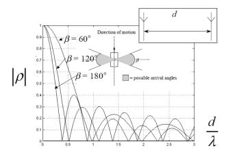
Figure 1. Correlation for two dipoles with changing inter-element spacing and three distinct angle of arrival [7].
