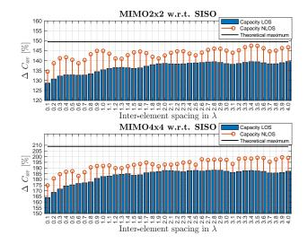
Figure 4. V2I channel capacity for different inter-element spacing for MIMO 2x2 and MIMO 4x4 with respect to the SISO channel capacity in percent and a fixed SNR of 10 dB.
