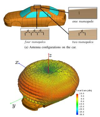
(b) Radiation pattern of a monopole mounted on the car rooftop.
