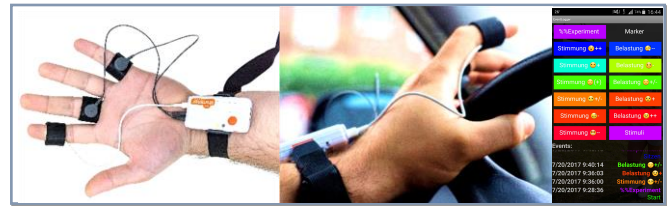
Figure 7. Experimentee with GSR electrodes and PGG fingertip sensor (left and middle); Event logger interface (right).
