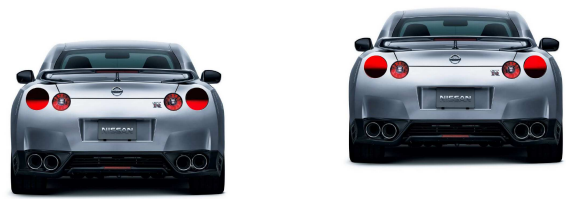
Figure 5. Modulated taillights showing transitions between ON and OFF, depending on the vertical position in the image
