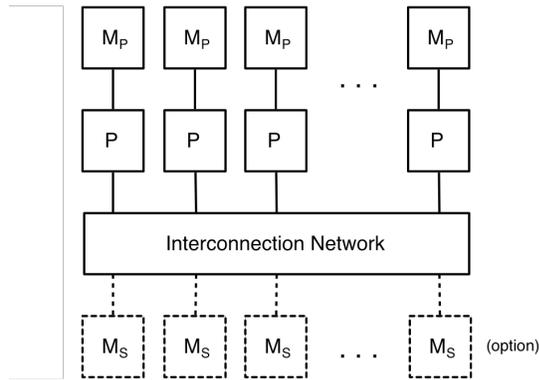
Figure 4. Block diagram of the resulting MPSoC Architecture.
