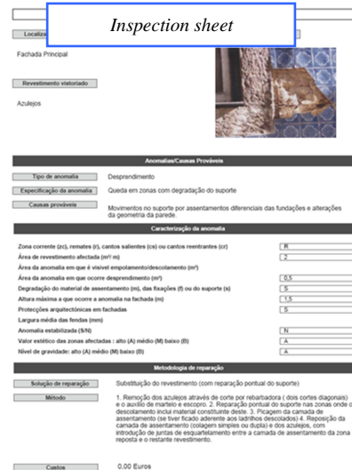
Figure 7: An inspection sheet report.
