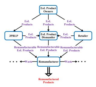
Figure 1. RL process for EoL product remanufacturing.
