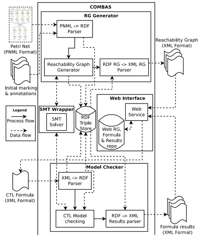
Figure 1. Architecture of the COMBAS model-checking framework.
