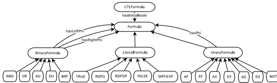
Figure 3. CTL formula ontology with parametric elements.
