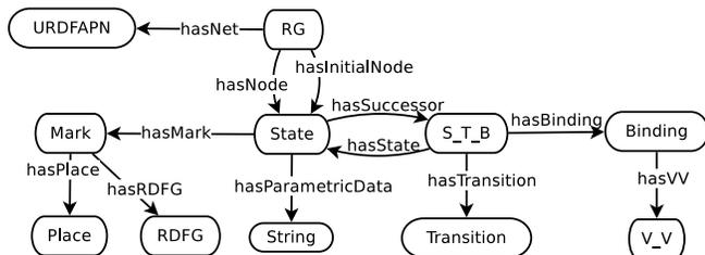
Figure 2. Ontology for the Parametric Reachability Graph.
