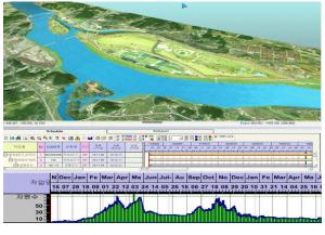
Figure 6. Prediction of flood levels using 4D CAD system
