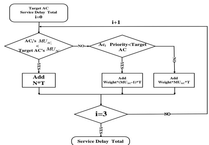
Figure 2. Flowchart for the computation of service delay.
