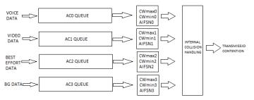
Figure 1. Demonstration of EDCA Mechanism
