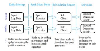
Figure 3. Overall high-level architecture of the index pipeline.
