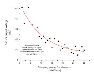
Figure 4. Theoretical results for the pyroelectric voltage at different incident electron energy values.
