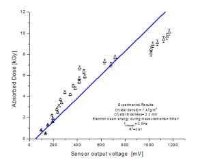
Figure 5. Calibration curve for the absorbed dose in the range of 0.5kGy to 10kGy, i.e., based on chopping frequency equal to 3.5 Hz and a 5MeV electron beam energy.
