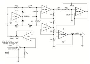
Figure 2. Electronic circuit for signal processing (resistors are in  $\Omega$  units).
