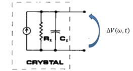
Figure 1. An equivalent circuit for the pyroelectric crystal, where  $R_x$  and  $C_x$  are the equivalent resistance and capacitance respectively.
