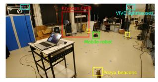
Figure 1. Experimental setup. One more Pozyx beacon is present but cannot be seen on this perspective.
