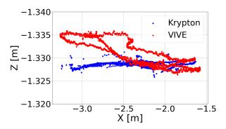
Figure 10. Side view of the HTC VIVE positioning results (red) alongside the Krypton CMM measurements (blue)
