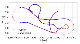
Figure 4. Marvelmind positioning results alongside Krypton CMM measurements.
