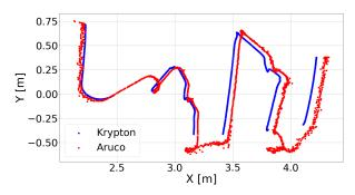
Figure 8. Camera positioning results (red) alongside Krypton CMM measurements (blue). Data was fitted to the left side of the figure, which is why deviation is smallest in this region. Evaluation is performed on the rest of the dataset which was not fitted.
