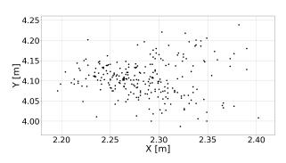
Figure 7. Reported positions by pozyx when the receiver remains static in an outdoor environment. Beacons were placed approximately 5 meters apart.
