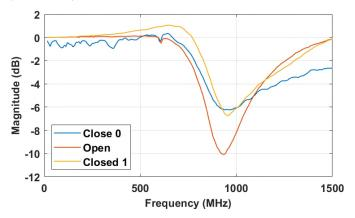
Figure 2. S<sub>11</sub> magnitude for open and close states. Close 0 corresponds to the first attemp of closing the button, followed by Open when the button is released and finally Close 1 when the button is pressed again.
