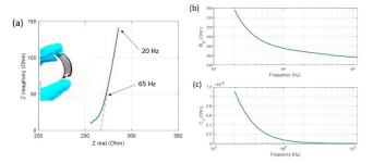
Figure 6. Electrochemical Impedance Spectroscopy (EIS) of the presented ECs. (a) Nyquist plot. (b) Equivalent resistance and (c) capacitance considering a simple model based on a  $R \parallel C$  circuit.
