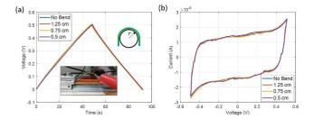
Figure 4. ECs performance under different bending conditions. (a) CC curves at the four different states ( $I = 1 \mu A$ ). Inset shows a bent EC, while the diagram depicts the definition of bend radius. (b) CV curves for the four bending states considered (s = 100 mV/s).
