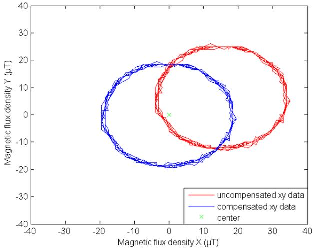
Figure 2. Shimmer sensor hard iron compensation
