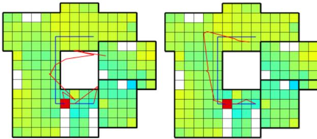
Figure 12: Suburban house route results for 3 components when room was not known (left) and when the room was known (right), blue line is the recorded route and red the estimated route.
