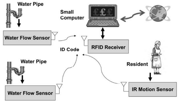
Figure 1. Functional block diagram of the monitoring system.
