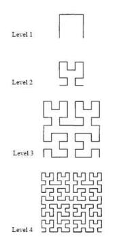
Fig. 3. The first 4 levels of Hilbert's curve in 2 dimensions
