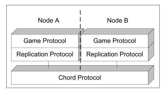
Fig. 1. Components of the simulation protocol stack
