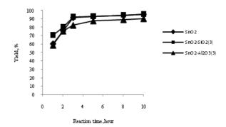
Figure 4. Effect of reaction time on FAME yield using  $SO_4^{2-}/SnO_2$  and its mixed metal oxide. Reaction condition: reaction temperature  $150^{\circ}C$ , methanol:oil ratio 10 for  $SO_4^{2-}/SnO_2$ -Al<sub>2</sub>O<sub>3</sub> (3), 15 for  $SO_4^{2-}/SnO_2$ -SiO<sub>2</sub> (3) and 30 for  $SO_4^{2-}/SnO_2$ , catalyst loading 6 wt % for  $SO_4^{2-}/SnO_2$  and 3 wt % for  $SO_4^{2-}/SnO_2$ -SiO<sub>2</sub> (3) and 30 for  $SO_4^{2-}/SnO_2$ -SiO<sub>2</sub> (3).
