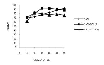
Figure 3. Effect of methanol to oil ratio on FAME yield using  $SO_4^{2/}SnO_2$  and its sulfated mixed metal oxide. Reaction condition: reaction temperature 150°C, catalyst loading 6 wt % for  $SO_4^{2-}/SnO_2$  and 3 wt % for  $SO_4^{2-}/SnO_2$ -SiO<sub>2</sub>(3) and  $SO_4^{2-}/SnO_2$ -Al<sub>2</sub>O<sub>3</sub>(3), reaction time 3 hours.
