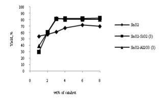
Figure 2. Effect of catalyst loading on FAME yield using  $SO_4^{22}/SnO_2$  and its sulfated mixed metal oxide. Reaction condition: reaction temperature 150°C, methanol:oil ratio 10, reaction time 3 hours.
