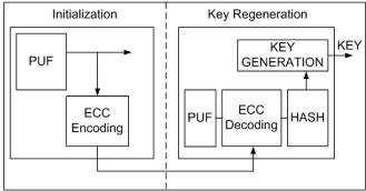
Figure 2. Key Generation Schematic with Conventional RO-PUFs.
