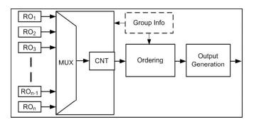
Figure 3. Block Structure of Ordering Based RO-PUFs.
