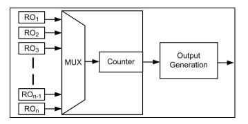
Figure 1. Block Structure of Conventional RO-PUFs.
