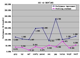
Figure 10. The relationship between performance improvement and profiling overhead of CrossBit compared with the natively translated code from MIPS-*x*86.
