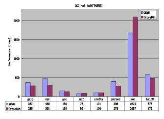
Figure 7. Performance comparison of the CrossBit with QEMU. The bars represent the time (sec) consumed by them from translating *x*86-POWER (shorter is better).
