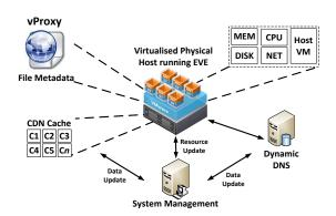
Fig. 3: Components of an Elastic Video Endpoint
