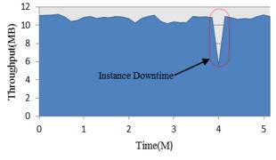
Figure 7. The Throughput of the Network during Instance Migration
