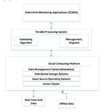
Figure 6. Cloud Computing framework for Smart Grid Monitoring Application
