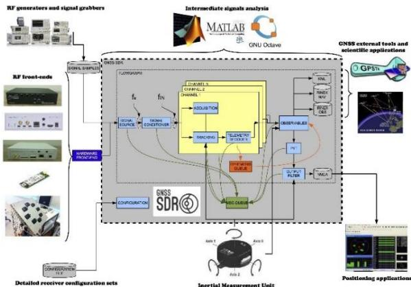
Figure 1 - Overview Software-Defined Radio GNSS-SDR [19].
