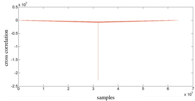
Figure 8. Cross correlation between the original and recovered chirp signals.
