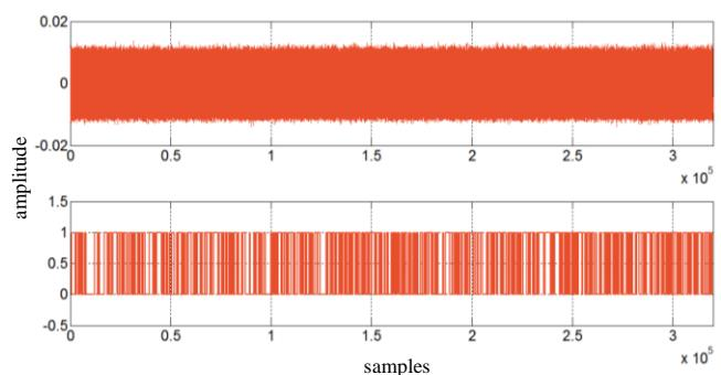
Figure 10. GPS signal mixed to interference and demodulated.
