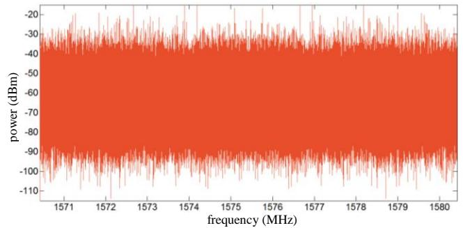
Figure 4. Spectrum chirp signal (interference signal).
