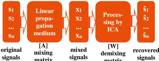
Figure 1. Block diagram of the ICA.
