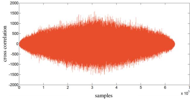
Figure 6. Cross correlation between the original chirp signal and the recovered GPS signal.
