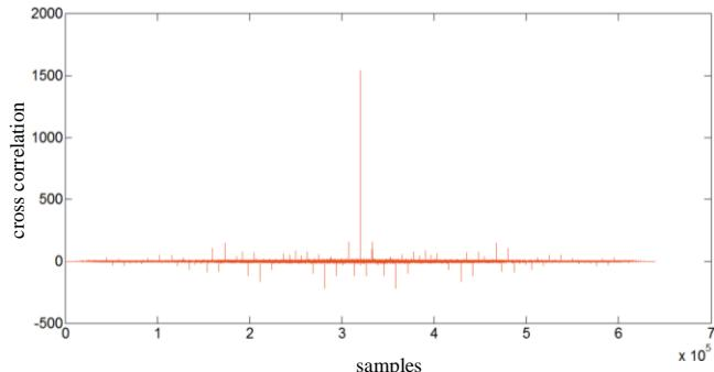
Figure 7. Cross correlation between the original and the recovered GPS signals.
