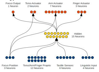
Figure 2. The architecture of the robot's neural controller during the first training phase. The neurons are grouped in clusters. Arrows between two clusters indicate full connectivity between the two corresponding groups of neurons.
