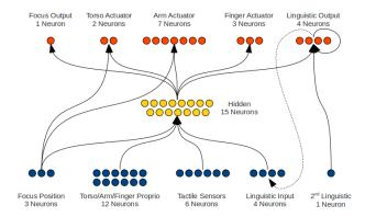
Figure 5. The architecture of the robot's neural controller during the second training phase (ST and LST conditions).
