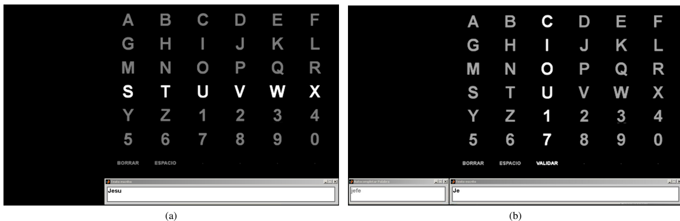
Figure 3. The interfaces of the two 7 x 6 matrix spellers that were tested: the Spellermod (a) and the SpellermodPred (b). The Spellermod presented a 7 x 6 virtual keyboard and a text box for displaying the user’s message, whereas the SpellermodPred showed an additional text box for displaying the word suggested by the word predictor.
